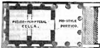
FIG. 12.—So-called Temple of Fortuna Virilis. The black shows tufa; the shading travertine.
